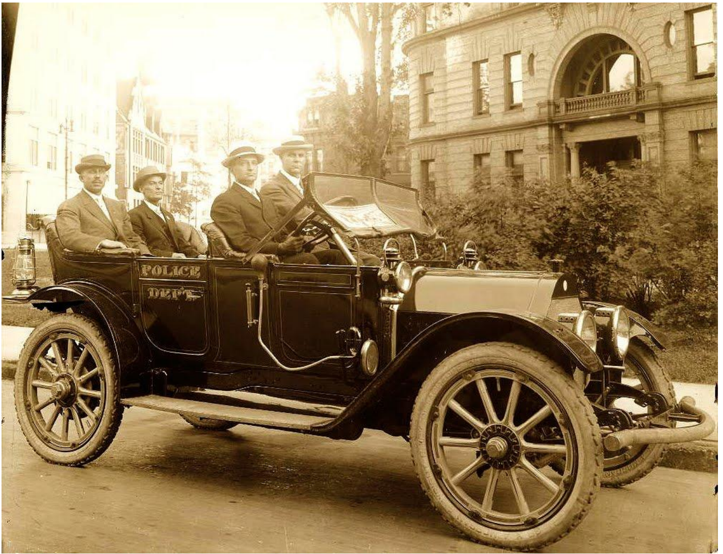
It looks like the Police department has a 1912 Chalmers model 10, 30 hp tourer. They're using a hurricane lamp tail light.
