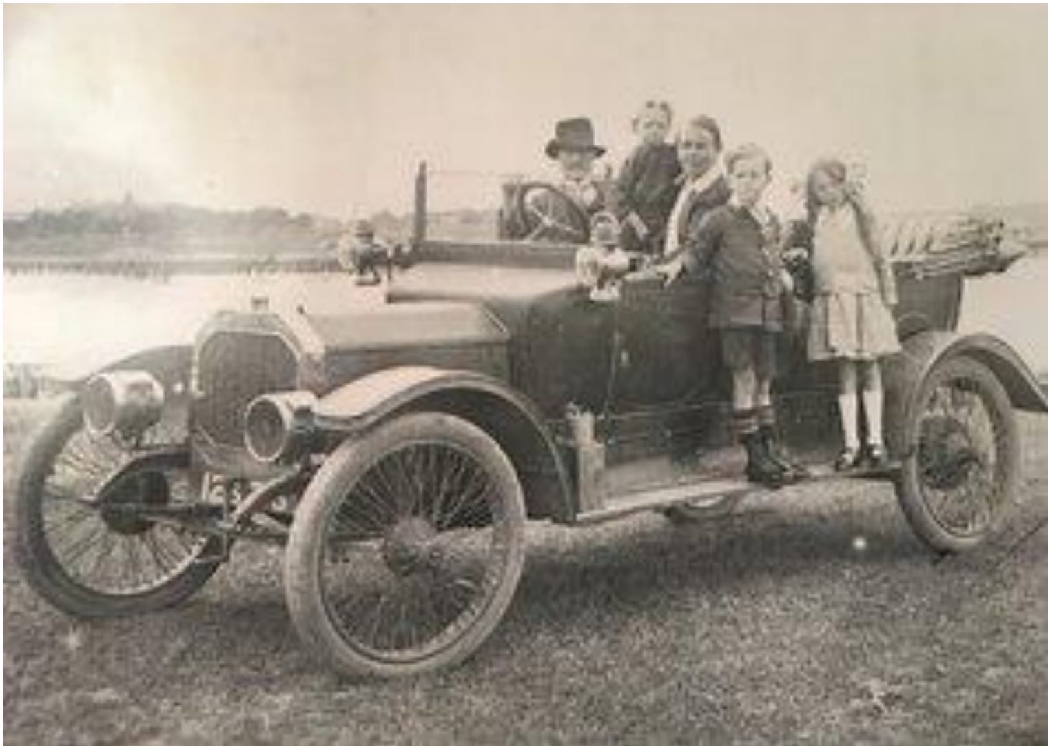
An Australian 13.9 hp BSA tourer. Beginning in 1912, BSA cars used all-steel bodies.
